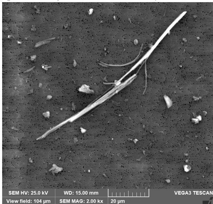
Figure 4. SEM Analysis of Asbestos Fibres in Air Samples.
